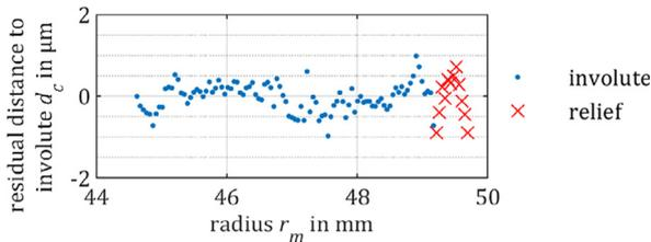
Fig. 4. Result of the automatic partitioning of the holistic approximation for real measurement data with the residual orthogonal distances  $d_c$  to the crowned involute and the tip relief, respectively. The standard deviation is 0.34  $\mu\text{m}$  for the involute residuals and 0.53  $\mu\text{m}$  for the relief residuals.
