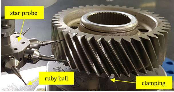
Fig. 3. Tactile measurements on a helical gear with modified flanks using a star probe with 1.0 mm diameter ruby balls.
