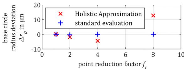
Fig. 6. Base circle radius deviations  $\Delta r_b$  caused by evaluating a reduced number of points (point reduction factor  $f_r$ ) compared for standard evaluation and holistic approximation.)
