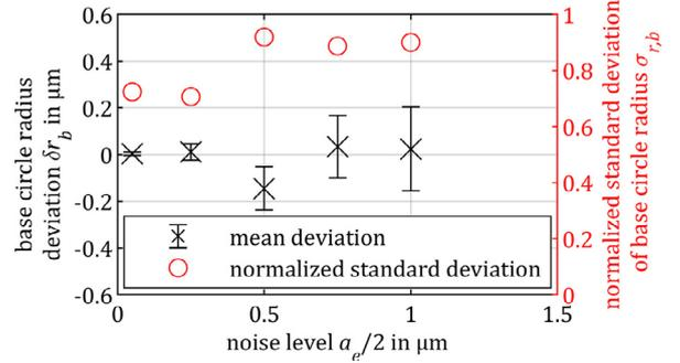
Fig. 5. Mean base circle radius deviations  $\delta r_b$  of 100 repeated simulations over the level  $a_e/2$  of equally distributed noise as position measurement noise (the error bars represent the standard error) together with the normalized standard deviation  $\sigma_{r,b}$  of the approximated base circle radii, normalized by the range  $a_e$  of the position measurement noise.
